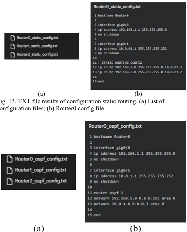
Fig. 14. Ospf configuration results txt file. (a) List of configuration files; (b) Router0 OSPF config file.
